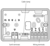
The TRTD7 is supplied with a standard back box, which can be used if there is no existing back box already installed. The new back box may be screwed to the wall using the fittings provided.
