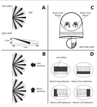
To restrict the sensor coverage, preventing detection in unwanted areas, mask the sensor lens using the masking label provided (see diagram D). The top section of the lens covers long range detection, the bottom covers short range. Similarly the left and right lens sections cover the left and right detection areas respectively.
