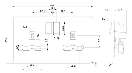
Ideal upgrade to existing double switched sockets around the home. 13A rated with DP switch.
