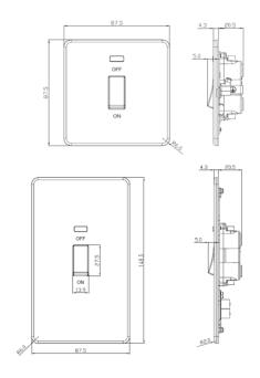
Cooker control units enable isolation of the unit so that maintenance and repairs can be carried out separately. The unit can be switched off, preventing the appliance from being turned on accidentally - for example whilst cleaning. Control two or more cooking appliances in the same room, providing rating is sufficient.
