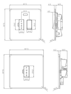
Fused spur units or connection units are an electrical switch with a built in fuse, designed for appliances that do not have or require a fused plug top. Fused spur units are also used for high powered electrical equipment with heavy continuous load, so that the appliance can be isolated by a single cable from a ring main for safety and maintenance purposes. 13A rated available with and without a double pole switch/neon.
