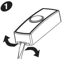
Using a small flat screwdriver, insert into the locking clip and gently twist. The back plate will unclip from the Bell Push.
