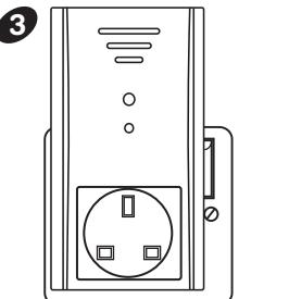
Insert the Plug-in Chime into a standard 220-240V ~50Hz wall socket and switch the socket ON, **Chime will ring**.
