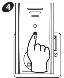
Press the learn button (L) on the front of the Chime to enter the Learn mode. **The chime will ring to confirm.**
