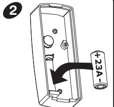
Insert the 23A battery (supplied) into the battery holder, making sure the Positive/Negative terminals match the internal markings. **Battery Comes Preinstalled**
