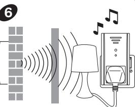
Test the Chime in the intended location, as internal walls and surfaces may reduce operating range. DO NOT mount onto metallic surfaces.
