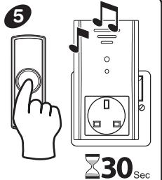
Press the Bell Push within 30 seconds, **the Chime will ring to confirm that the Bell Push has been paired to the Chime.**
